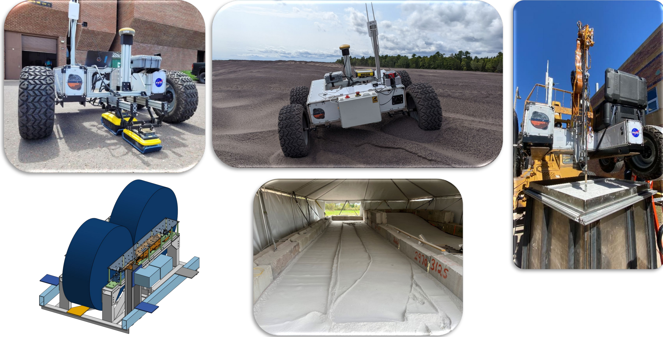
Figure 4: Field testing with field rover (HOPLITE) with the LuSTR20 PHCP and GPR measuring properties down to 1 m depth. Wheel durability (26k km at -196C) and traction testing on flat and sloped terrain was done for LTV prototype development.
