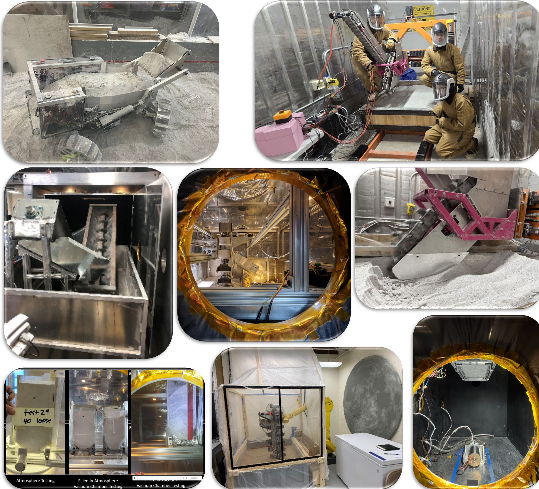
Figure 2: Various excavation robotics and technologies testing are shown here for granular regolith, icy regolith and ice-cemented regolith. Long duration testing (15 days+) is performed in DTVAC, sometimes at Cryo temperatures. Dust exposure and thermal cycle testing is performed under vacuum and cryo/hot conditions.
