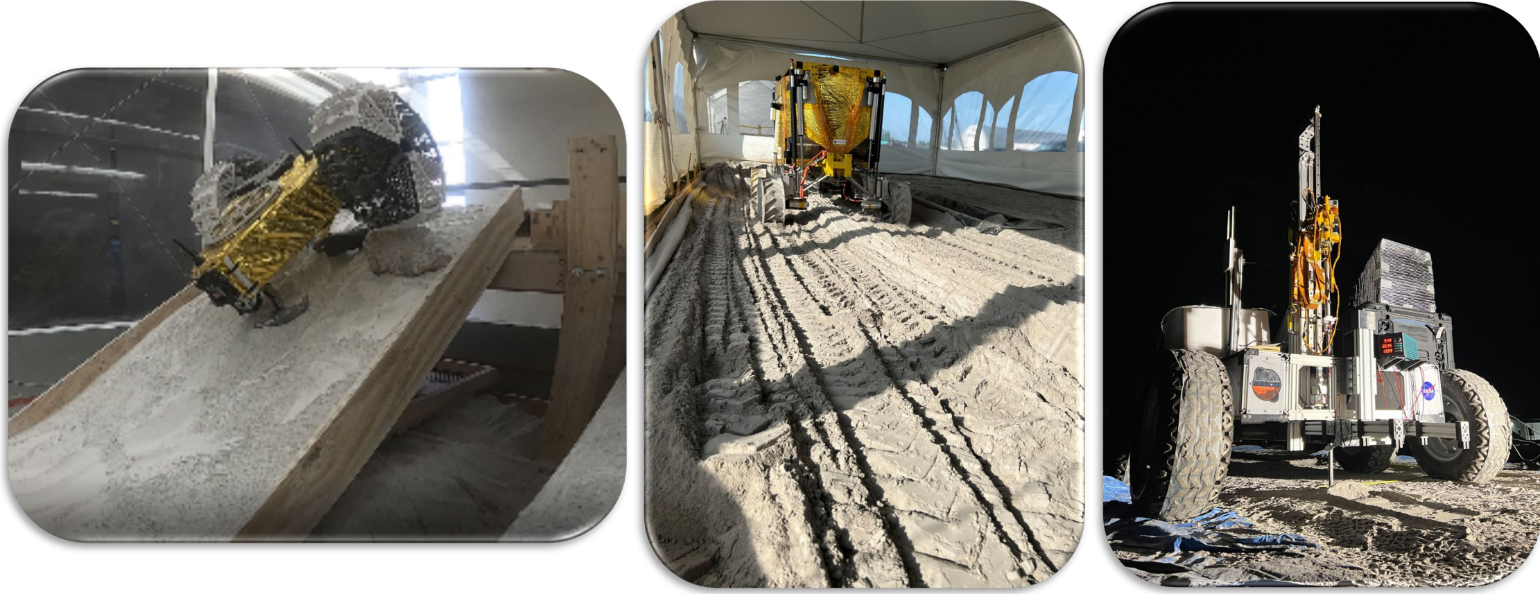
Figure 1: The T-REX rover (Left) demonstrating superconducting cable deployment while descending into a crater, the PRIMROSE rover (center) as part of the NASA Break the Ice Challenge and the LuSTR20 PHCP project (right).
