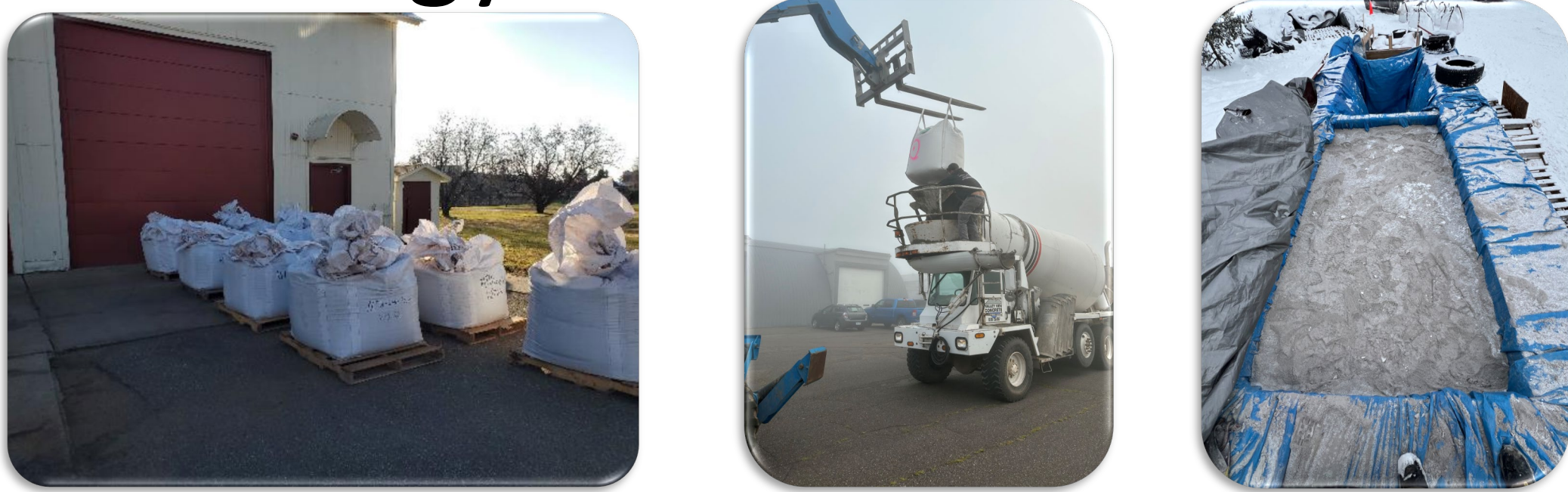
Figure 3: Regolith mixing for the trench testing for the LuSTR20 integrated culminating field test of the cone penetrometer and ground penetrating radar. Up to 30,000 kg of lunar simulant is available for creating testbeds as desired.
